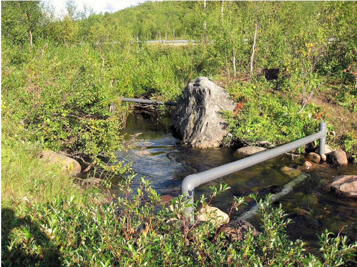
Figure 25. The stationary antennas in Vuolit Vedis that monitored the movement of tagged salmon parr into and out of the stream.
