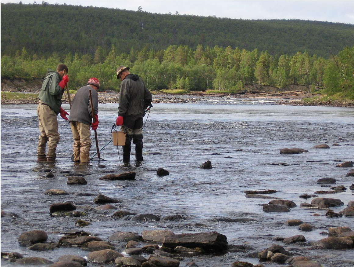
Figure 2. The electrofishing surveys in the tributaries of the River Teno were conducted by a three person team, including the user of the anode and two persons collecting the stunned fish with dipnets. Photo: A. Mäki-Petäys.
